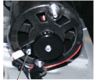
Speed Sensor on Main Drive Motor
