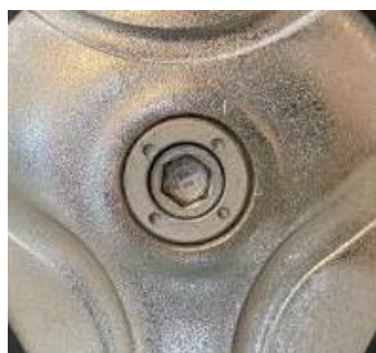
Figure 7 - Original, Fast Disassembly Screw
