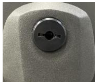
Figure 8 - Replacement Screw Requiring Crank Puller
