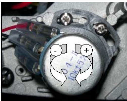
Figure 5 Lift motor potentiometer adjustment and how it affects on readout value
