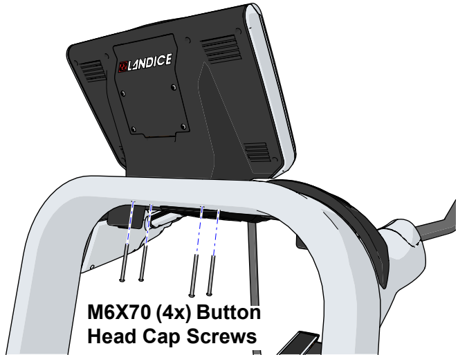
Figure 2-19. Console Assembly Bolts
