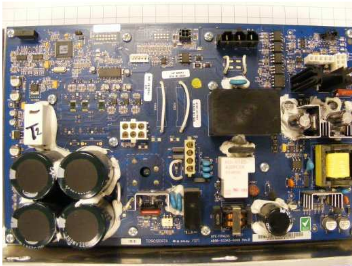
A DSP motor controller
