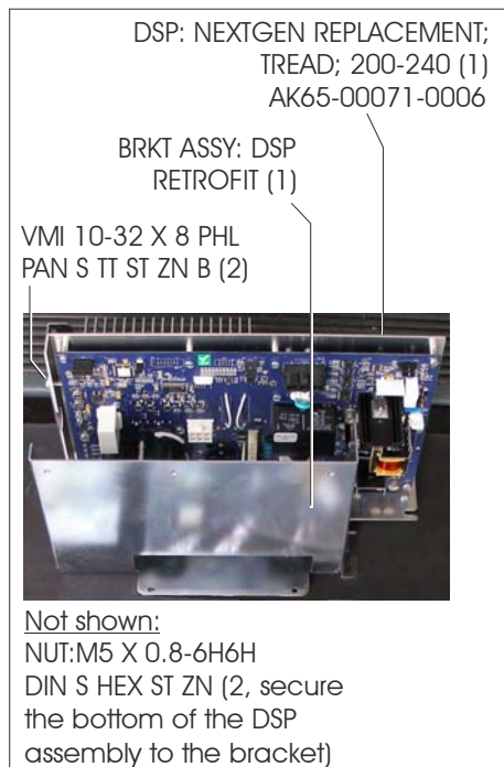
Fig. 4: 230V DSP Retrofit Bracket Assembly
