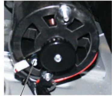
Speed Sensor on Main Drive Motor
