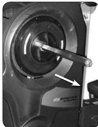
Figure 10d - Location of long screw to secure shroud
