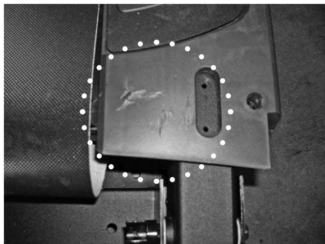
Figure 15: Damage caused to treadle by rear step if not covered.
