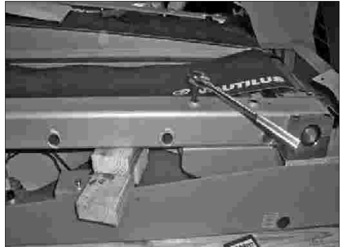
Figure 5: Brace treadles with wooden blocks.
