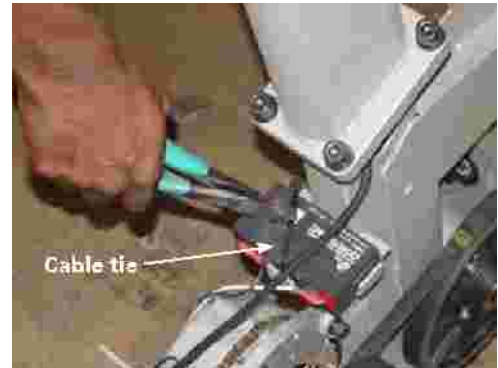
Figure 11 - Cut cable tie
