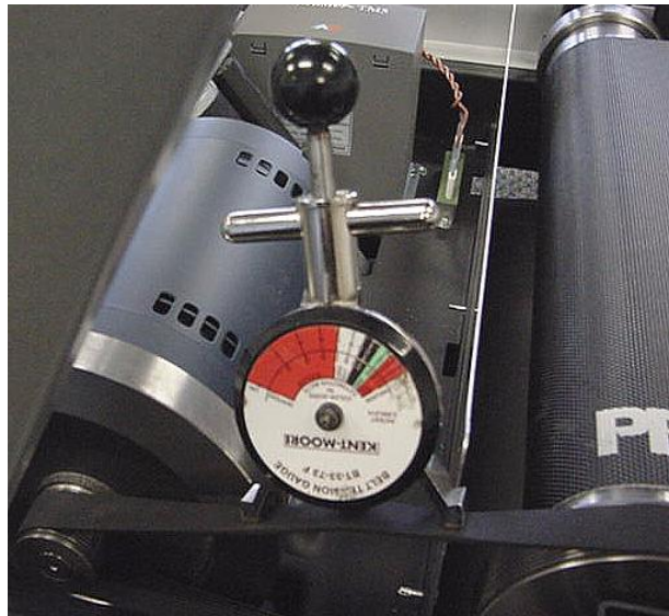
Diagram 8.2.1 - Drive Belt Tension Gauge
