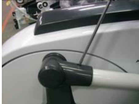
Step2: If has gap and noise please do repair procedure, use a Phillips screwdriver to open fix Pedal Arm Cover-Top bolt and remove.
