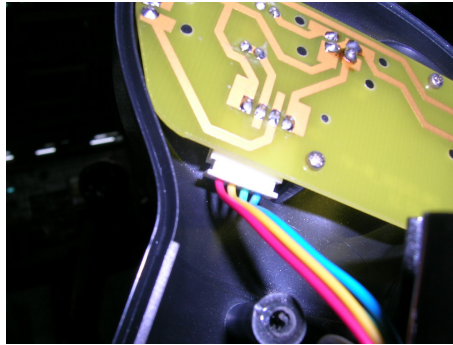
Step 2: Plug in 4pin.
