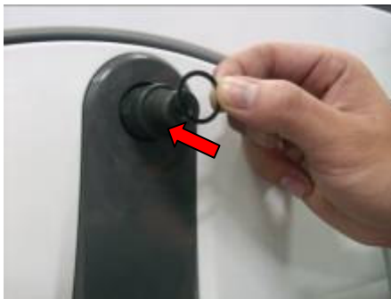
Step7: Then take a 22X17X1mm washer to cover crank big pivot.
