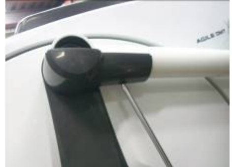
Step3: Then also use a Phillips screwdriver to open fix Pedal Arm Cover-bottom bolt and remove.
