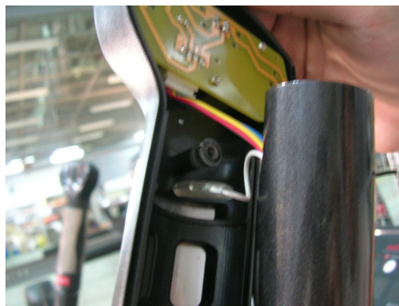
Step 5: Arrange the wire and to install handle bar tube.
