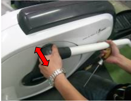
Step1: First use both hands to move both pedal arm cranks check have gap and noise.
