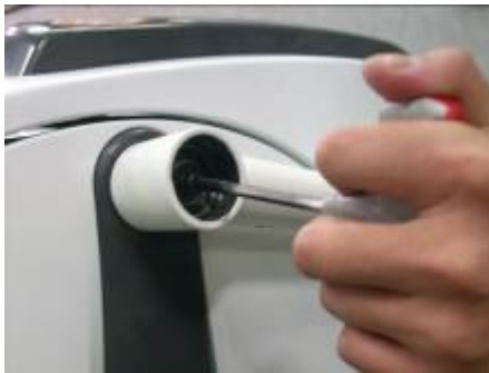
Step4: Use a 5mm Hex wrench to open fix pedal arm bolt .
