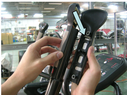
Step 7: Then install rear cover.
