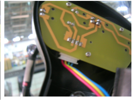
Step 3: Confirm 4pin at PC board well.
