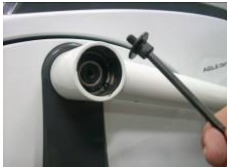
Step5: Remove both bolt and washer.
