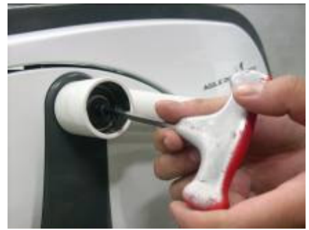
Step9: Use 5mm Hex wrench screw in both washer and bolt.
