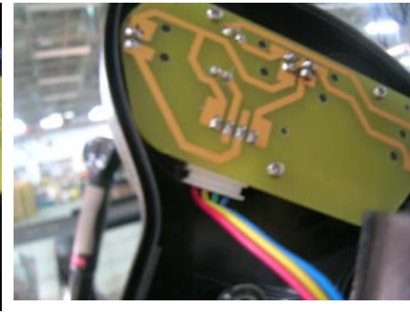
Step 3: Confirm 4pin at PC board well.
