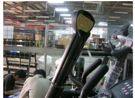
Step 6: Confirm front cover at handle bar tube very well.
