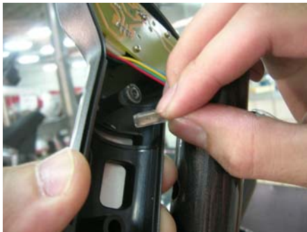
Step 4: Connect hand pulse sensor plug at front cover .
