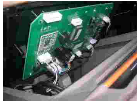
Step 3: Carefully lift up the with console main PCB plastic insert from console upper plastic cover.
