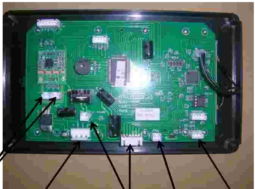
Step 4: Carefully use hand disconnect All connector on the main PCB.
