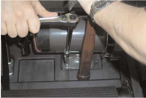
Figure 13: Poly V Belt Tension Adjustment
