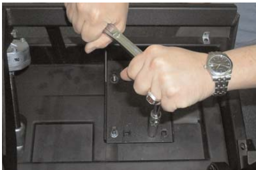
Figure 11: Lock Bolts on Motor Bracket
