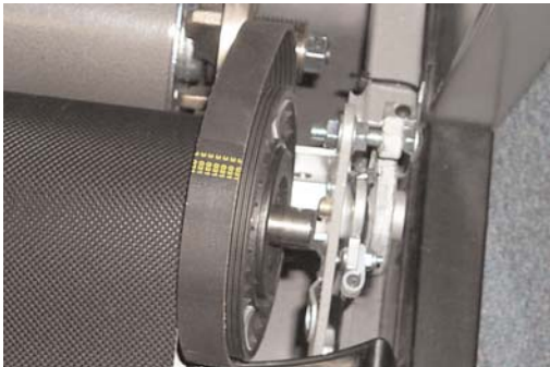
Figure 11: Slide New Roller In Position
