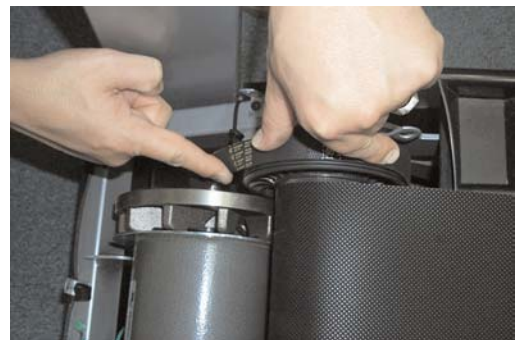
Figure 6: Remove Drive Belt
