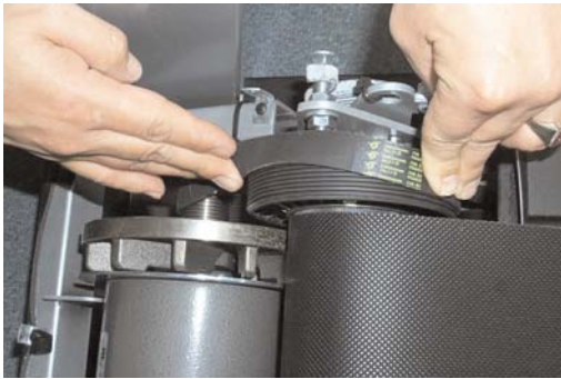
Figure 7: Remove Drive Belt (continued)
