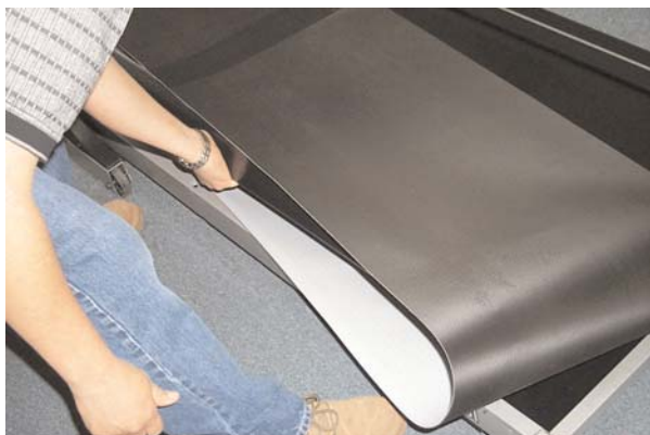
Figure 3: Remove Old Walking Belt
