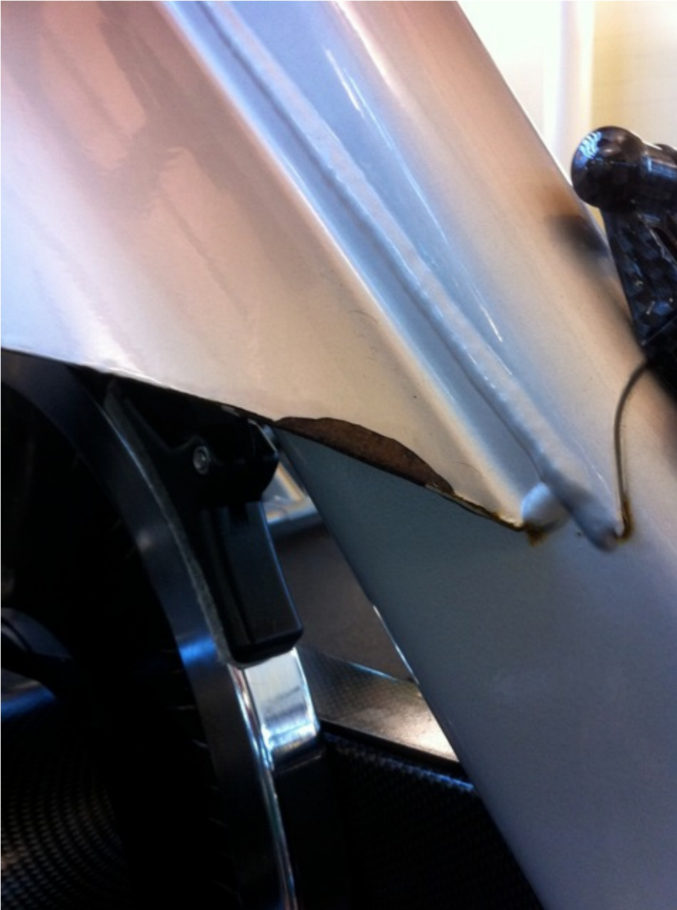
Worst Case Rust
